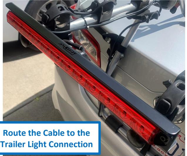
3. Route the cable along length of the rack to the vehicle connection and use cable ties to secure the cable to the rack frame. Bike racks have many pivot points. Be sure to route the cable away from and around pivots to keep them from getting pinched.
