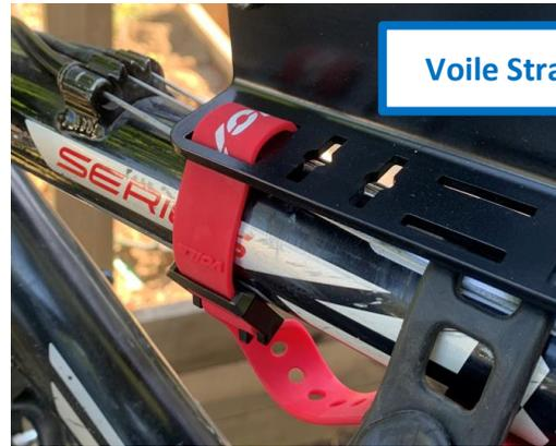
2. If you're attaching the light to a delicate surface install a section of the provided sticky back Neoprene on the bottom of the light. The Neoprene also provides a non-slip surface to improve installation.
