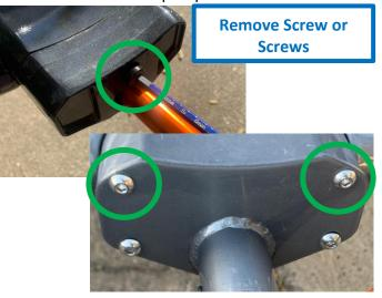
3. Place light on rack end and install single M12 screw or provided longer ¼-20 screws on NV 1.0 through the bracket and into the end of the rack.
