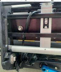
Route cable along rack and test the light.
