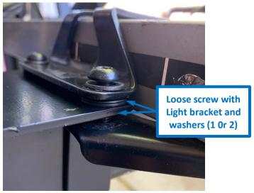
4. Install the rear most screws with washers (provided) between the light bracket and the upper rack bracket. Tighten all four screws evenly to clamp the light and tray in place while keeping the light centered on the frame.
