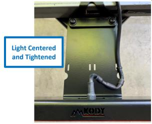
6. Route cable along the length of the bike rack and secure with the provided cable ties. Bike racks have many pivot points. Be sure to route the cable away from and around pivots to keep them from getting pinched.
