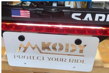
3. Install longer screws through the light, the light bracket and license plate bracket with both washer and install the nut onto the screw. Tighten the screw into the nut until all parts are clamped well.
