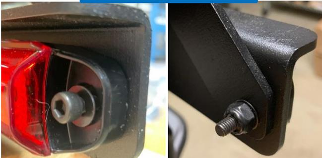
4. Install your license plate when needed into the threaded holes using the M6 screws or the thumb screws.
