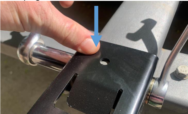
Hold bracket Down and Flush During Tightening
