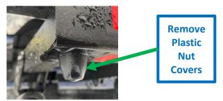
2. Remove two screws and nuts attaching the last tray to the bike rack.
