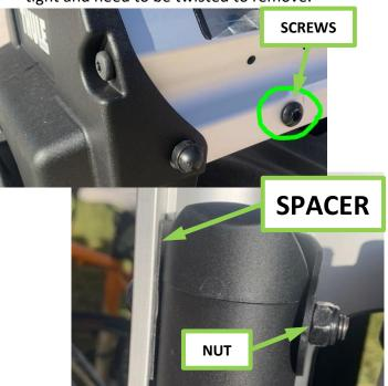
3. Set the bracket in place lining up the screw hole and open guide. Slide the bracket back, down, and then pull forward to engage the open guide onto the screw cap.
